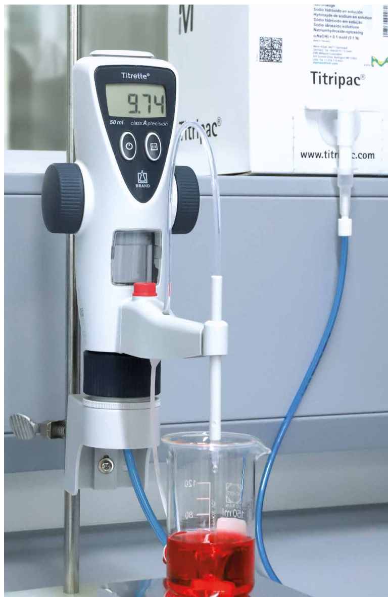
Titrette® extraction system for Bag-in-Box (Titripac® is a registered trademark of Merck KGaA, Darmstadt, Germany)
