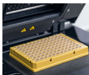
Thin-walled wells for reduced cycle times
